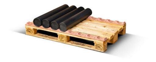
**2.** Once all rolls are placed on the first layer, fold 2 more cradle pairs for the second layer of rolls.
